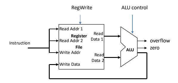
Note that Register File is not written every cycle (e.g., sw), so we need an explicit write control signal for the Register File
